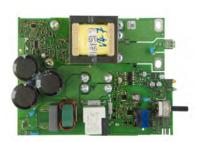
· Replacement circuit board for G17641 inverter welder
