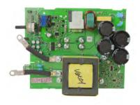
• Replacement circuit board for 200amp GYS inverter welders G18129
