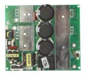
· Replacement inverter welder circuit board
